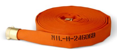
This double jacket municipal grade fire hose incorporates a lightweight polyurethane liner that meets all the requirements of NFPA 1961 and Mil Std. 24606. It is designed for use as an attack hand line hose and can be used for potable water transfer in an emergency
