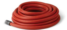
CONSTRUCTION: Polyester Single Jacket Polyurethane Lined Hose TEMPERATURE RANGE: -40F to 150F (-40C to 65C) COUPLINGS: NH Aluminum Couplings HOSE COLORS:
