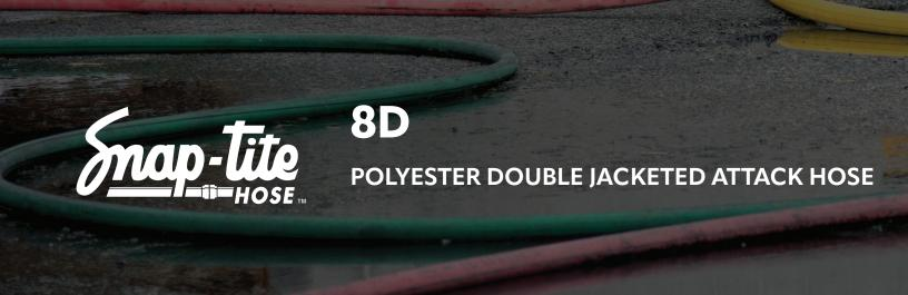
8D is a municipal grade double jacketed hose with a lightweight EPDM rubber liner that meets all the requirements of NFPA 1960. It is designed for use as an attack handline hose and is manufactured to a service test pressure of 400 psi (2758 kPa) to handle all fireground challenges with ease.
